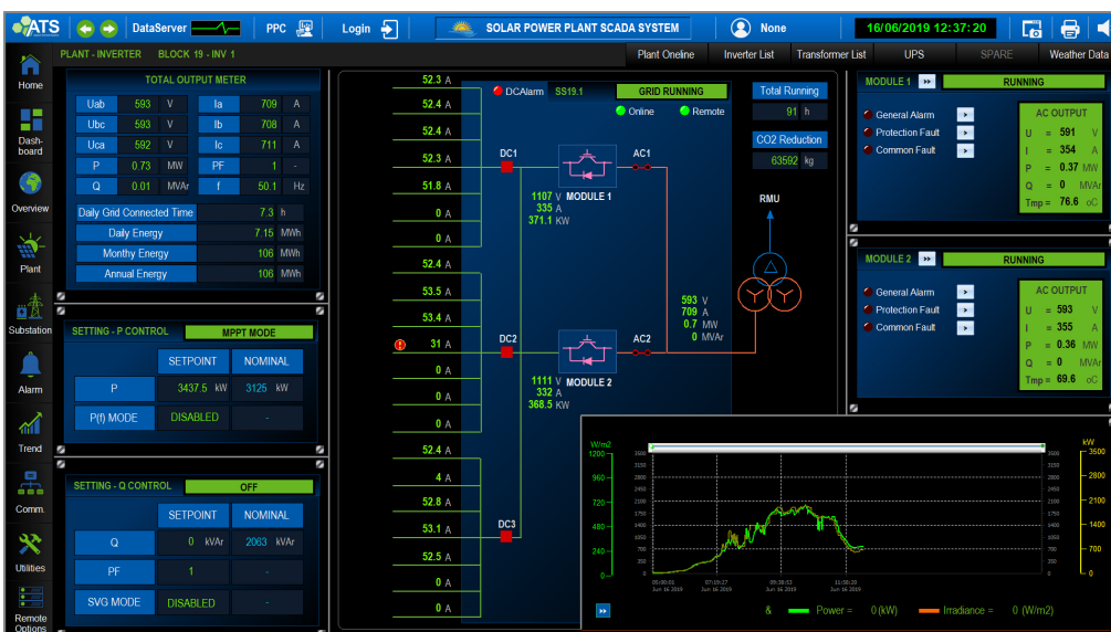
Figure 16. PV Inverter Data Monitoring and Control
