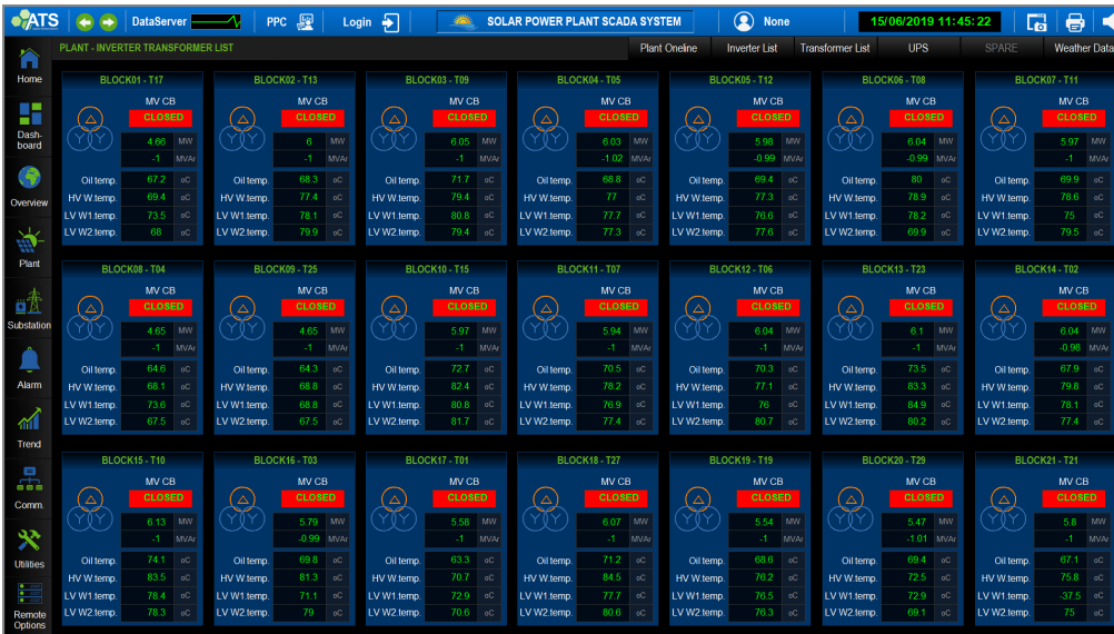
Figure 17. MV Transformer Monitoring
